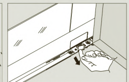
Press the locking device under drawer bottom and pull out the drawer
